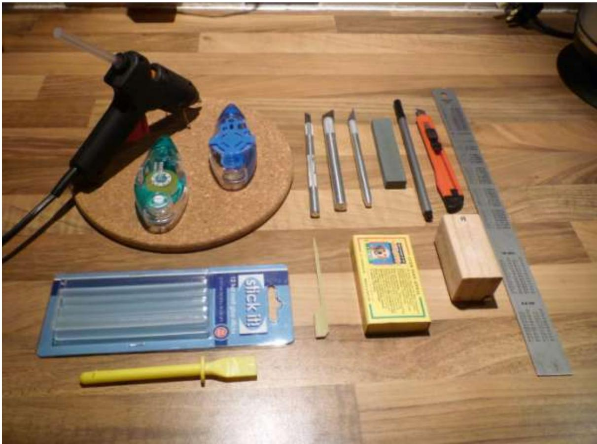
The list is (clockwise from top left): Cork heat mat, Glue gun 7mm (with modified tip, more later), Green Stix2 roller (removable), Blue Stix2 roller (permanent), scalpel x3 (various blades, but 1 with no.11 blade would be ideal), sharpening block, black fine tipped ink marker, craft knife, Steel rule, wooden block from child's building set, box of matches (for sanding), bamboo pick for making holes (anything round and sharp would do), Glue sticks, spreader (for wiping excess)
